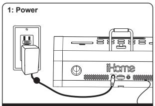
Attach AC adaptor cable to DC jack on back of the unit and plug the other end into a wall socket. Remove pull tab from the backup battery compartment on the bottom of the unit. Extend FM antenna for best reception.
